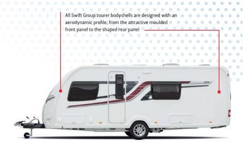
The latest pioneering SMART HT construction system from Swift Group features an entirely timberless bodyshell and is highly resilient to moisture
