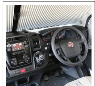
DASH FOR CONTROL Upgrades to the cab include automatic air-con, sat-nav and steering wheel-mounted controls for the stereo and hands-free phone
