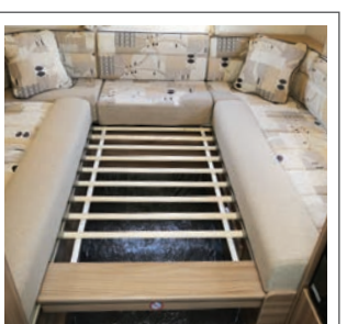
A DOUBLE? NO TROUBLE! Slide-out slats provide the support for the rear lounge's double bed. The whole assembly process takes a couple of minutes
