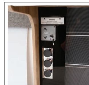
SAFETY IS THE KEY Controls for drop-down bed feature key operation as a fail-safe to prevent bed from being raised or lowered by curious little fingers
