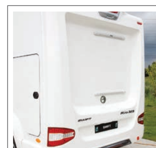
RAIL CONVENIENCE The single-piece GRP rear panel has rails for fitting a bike rack. When in transit, bicycles can be stowed in the rear garage
