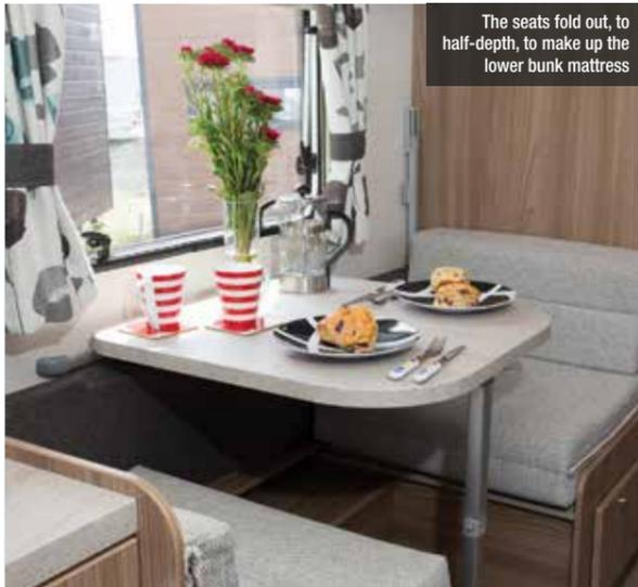
The seats fold out, to half-depth, to make up the lower bunk mattress
