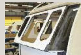
Structural Reaction Injection Moulding technology allows corners to be shaped
