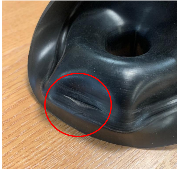
TJ0023 - Manufacturing fault
