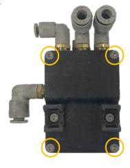
Once the cap has been removed. Remove the three rubber dampers, then tighten the 12 screws with a small Philips screwdriver. When re-assembling, apply a small amount of silicone to the rubber dampers and place them on the red circles, as shown in the picture. Then apply a small layer of silicone around the large cap to prevent any potential water damage, shown in the diagram on the right, then reattach the cover.
