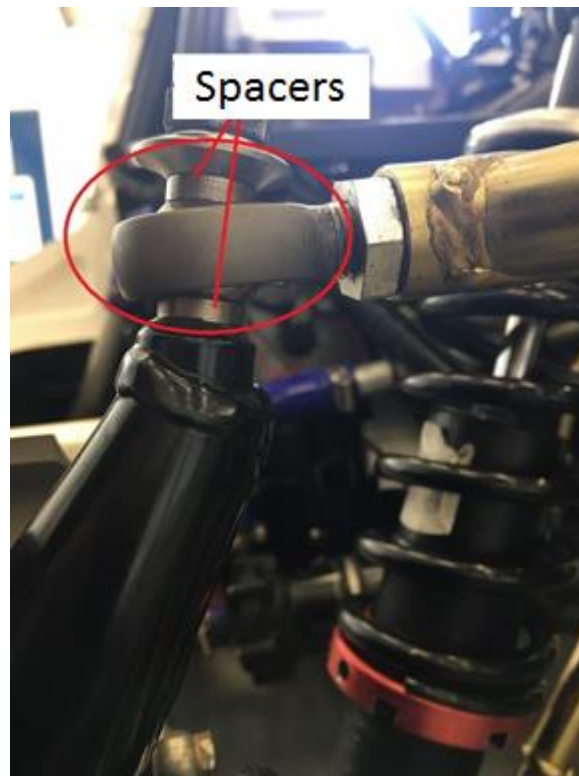
Figure 1 - Rear upright bolt with spacers
