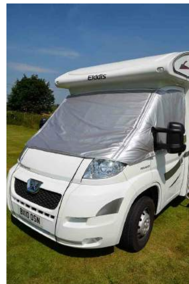
An insulated cover for the cab windscreen can help keep a motorhome snug, external type shown
