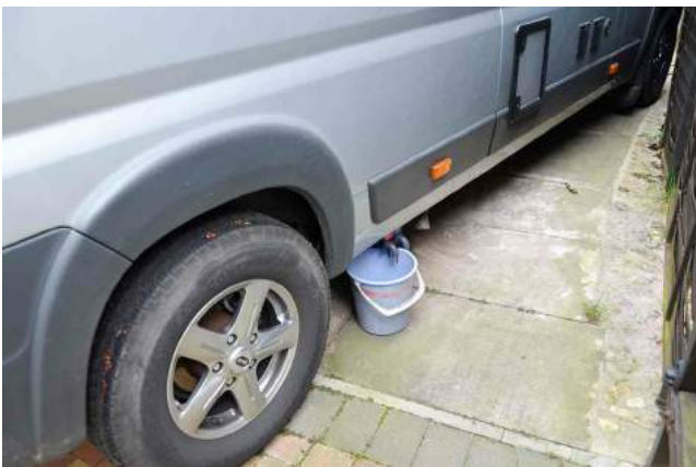
Draining to a bucket can help keep your waste tank from freezing up. It's easy to dispose of frozen waste from a bucket
