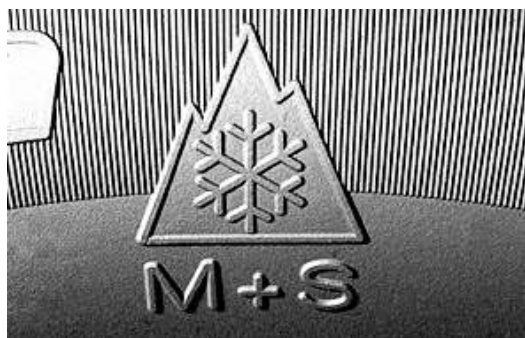
Winter tyres showing the three peaks and snowflake symbol can improve safety in winter but M+S or all-season tyres can help
