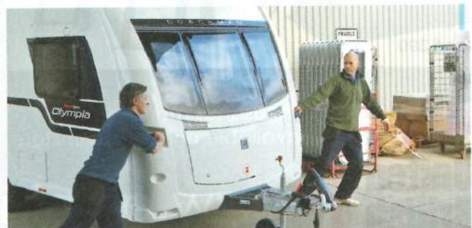
The van is then rolled off the line towards the test row, where all its components and utilities are fired up for several hours to check whether they're in full working condition before dispatch
