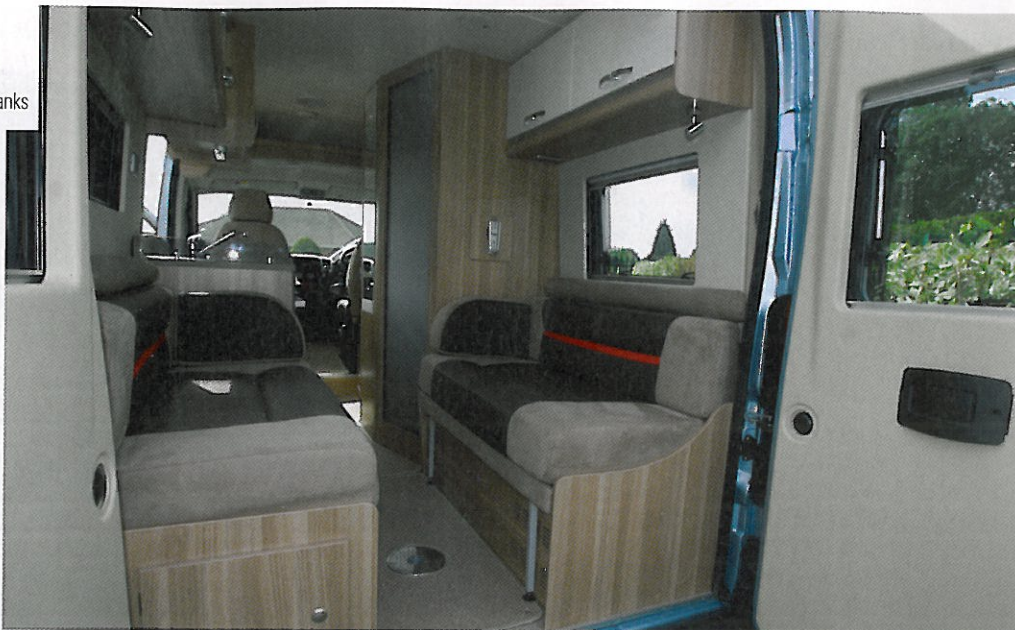
Automotive-style fabrics and the rear lounge layout from Rhythm squeezed into a 5.40-metre panel van (instead of 6.00 metres)
